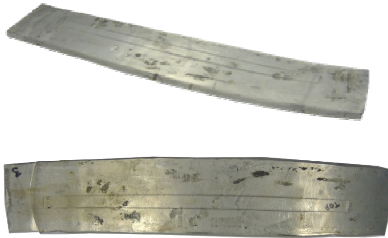
Figure 2 – Deformed specimen after rolling. The specimen is relatively straight and no detachment can be observed between insert and work-piece in both transverse and longitudinal direction.
