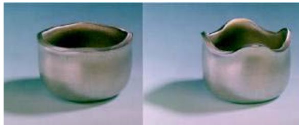
Figure 1 – ‘Earring’ of a cup after deep-drawing from a rolled sheet of aluminium (source http://aluminium.matter.org.uk )
